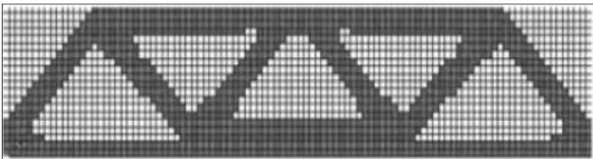
Fig. 1: Showing the MBB Beam using Independent Continuum Map Method Sui et al. [5].
